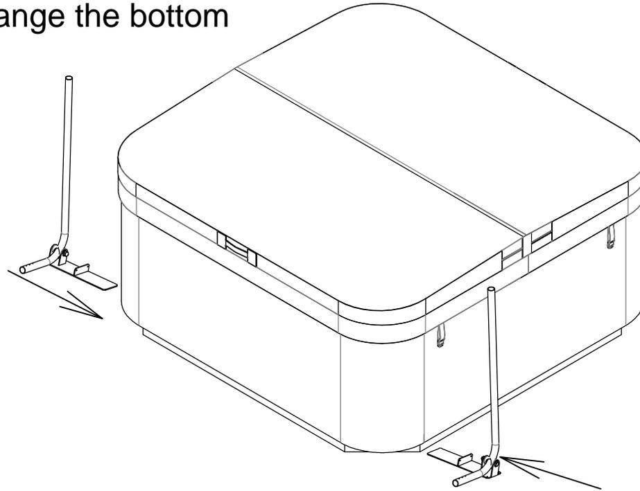
Installation steps Two: Install the stents on both sides respectively
