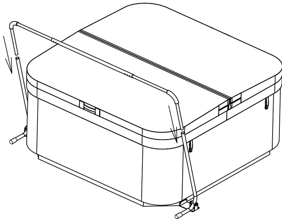
Installation steps five: Locate the lifter, and lock screws
