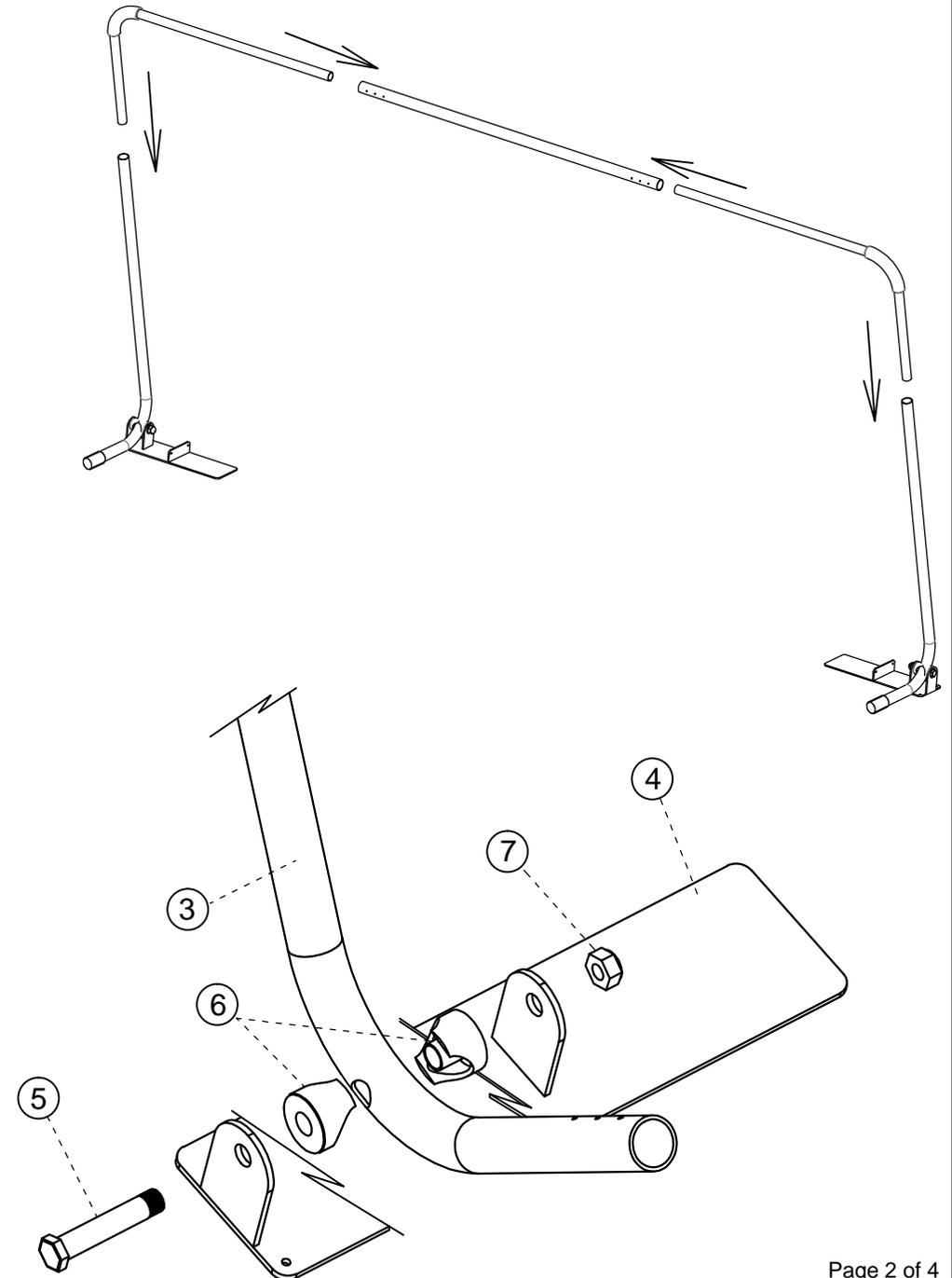
Installation steps One: Arrange the bottom position
